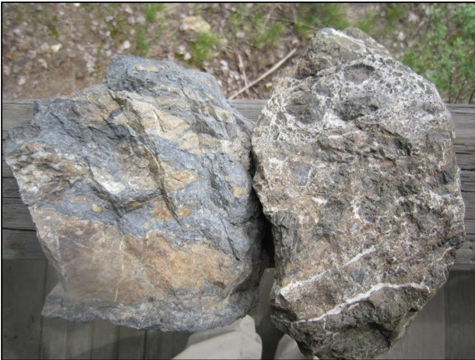
Photo 5: Samples of vein, taken from underground from the east extension of Level 4625; left sample shows fine-grained galena with remnant gangue, and right shows brecciated sphalerite-rich vein cut by quartz stringers.
